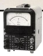
Fig. 3: An Advance Meters Advactype VM77 audio millivoltmeter, manufactured in 1953. It has a distinctive 'blood red' coloured front casing (see text).
