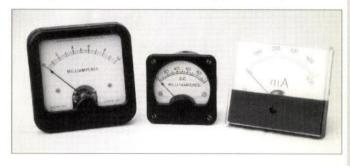
Fig. 5: A selection of useful surplus moving coil milliammeter (see text).
